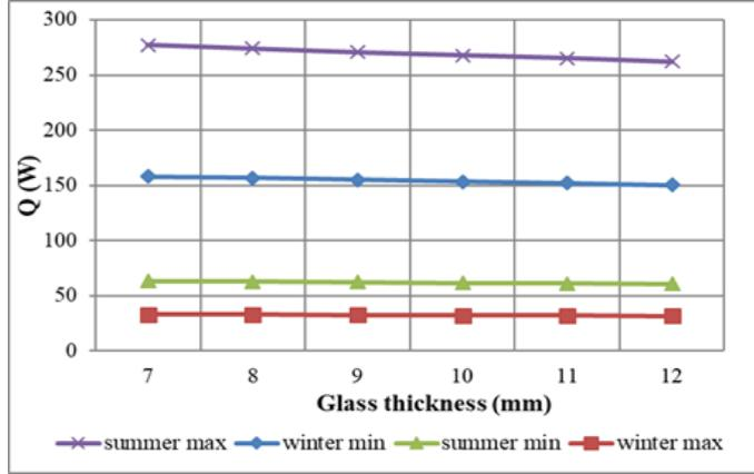
Figure 2. Heat flux through a single-glazed window with different glass thicknesses at different temperatures.
