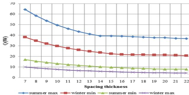
Figure 4. Heat flux through a double-glazed window with an Air filling at different spacing thicknesses and temperatures.
