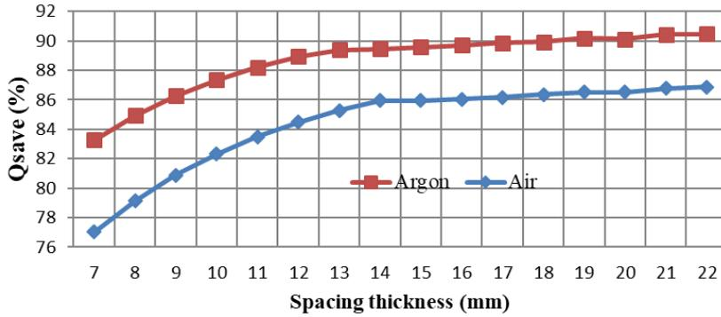
Figure 8. Heat saved when a double glaze window was used instead of a single glaze window.
