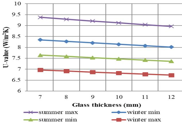
Figure 3. U-value for a single-glazed window at different glass thicknesses and different temperatures.
