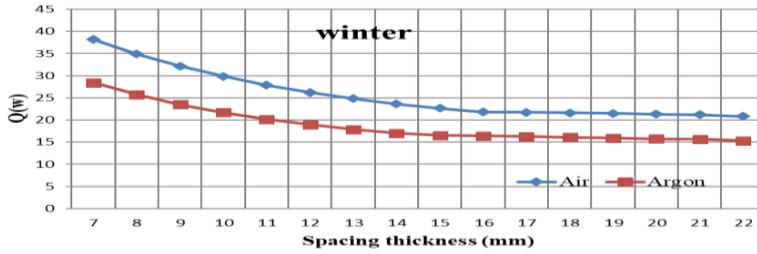
Figure 5. Heat flux through a double-glazed window with different spacing thicknesses and different gas fillings (winter).
