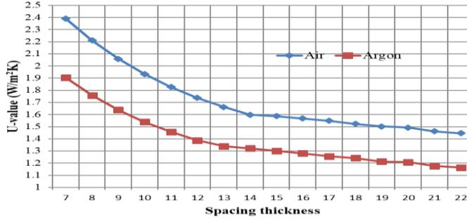
Figure 7. U-value for double-glazed windows with Air and Argon gases.
