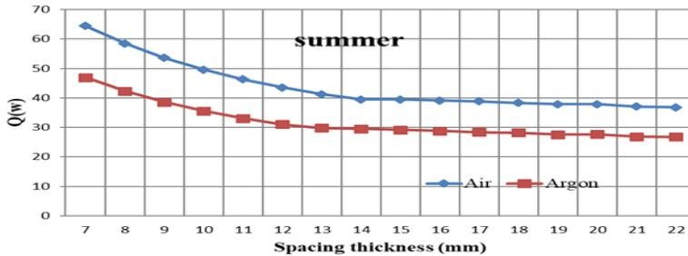
Figure 6. Heat flux through a double-glazed window with different spacing thicknesses and different gas fillings (summer).
